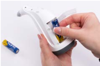
Figure 4 – Changing batteries: Remove battery on left
