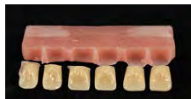
Figure 15 b: Fracture pattern; tooth base was not surface-conditioned
