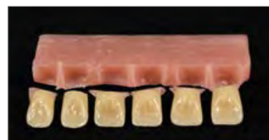
Figure 15 d: Fracture pattern; tooth base was only coated with bonding agent
